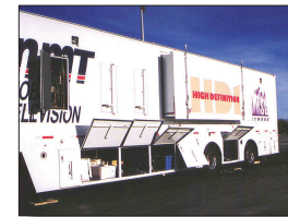
Figure 2.73 The truck above, one of NMT's high-definition trucks, is a double expando. Besides an expansion area that expands out the other side, a smaller expando section on this side of the trailer slides out and holds the monitor wall in the production compartment in order to provide more working space. The bays below house equipment, cable, manuals and spare parts. (Source: Tim Stoffel)
