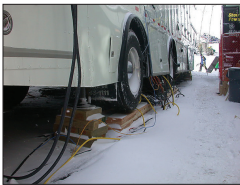
Figure 2.68 Snow and ice make the task of parking much more difficult. There was an incident a few years ago where a 48-foot trailer left overnight at Rich Stadium in Buffalo, NY with wheels blocked and tractor brakes on, slid down a slight incline and into a gate because of ice. (Source: Jason Taubman)
