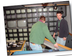
Figure 2.72 The truck engineers then move the stowed part of the front production desk into place.
