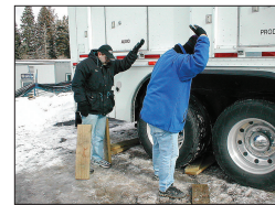
Figure 2.64 While smaller television production vehicles such as ENG and SNG trucks can have automatic leveling systems, there are no such systems for trailers that can weigh almost 80,000 lbs. Trailers are often carefully backed onto wood planks in an effort to level them. (Source: John Tomlinson — NEP)
